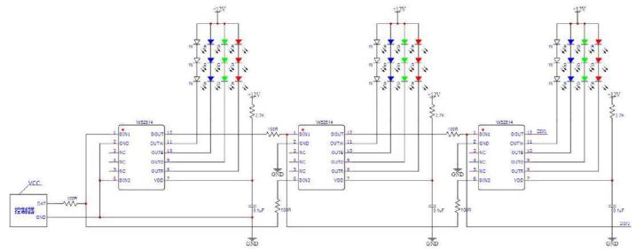
2. Supply voltage=24V(Each channel drives 6LEDs)
